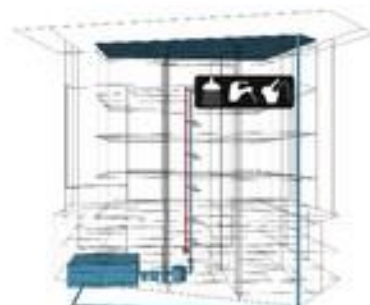
RAINWATER COLLECTION 100% DEMAND MET ON SITE 50,000 GALLON CISTERN
